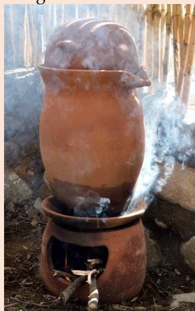
Replicas of the apparatus composed by a double rimmed jar and cover, on a fire-pot distilling laurel.
