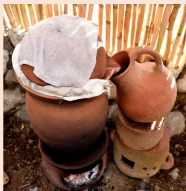
Replicas of the apparatus composed by a double rimmed jar and cover, on a fire-pot distilling laurel.
