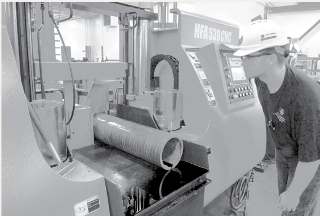
Precision cutting hollow bar on one of our Amada CNC controlled fully automatic horizontal band saws.
