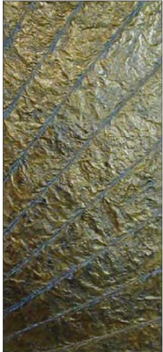
Figure IV-16. JT Cooper Studios creatively used brazing alloy to create texture and decorative seams for this door.
