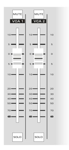
The 12 VCA master faders are fitted centrally in the console fader section below the audio Sub-Group output modules. Each VCA master fader has an associated Mute and Solo switch.
