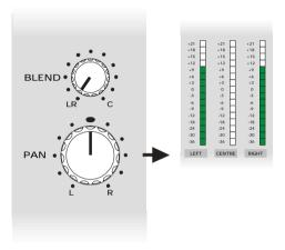
With Blend set in the fully clockwise position only the Centre bus is fed.
