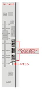
Then, to view or edit midi message settings, depress the SET switch on the relevant Aztec Input channel. The active MIDI channel number (0-15) is shown in the 7-segment display and this can be modified using the UP↑ and DOWN↓ keys.
