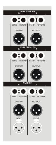
Aztec Sub-Group output module connections are arranged on a single panel along with those for the Master module and Stereo Auxiliary module interfaces.
