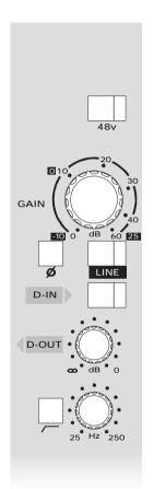
48v enables phantom powering. A master isolator is provided on the rear connector panel.
