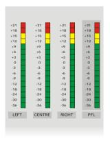
Solo'd AFL signals are metered on the L, C. R Master module LED bargraph displays. PFL has a dedicated bargraph display.
