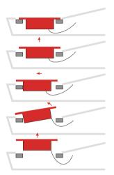
After removing these screws carefully lift the panel by ~20mm then pull it forward slightly being careful to avoid damage to the isolate switch at the front edge of the module.
