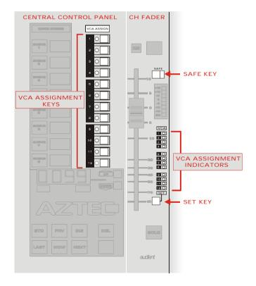
The stored assignment is displayed on the column of 12 LEDs adjacent to each channel fader.
