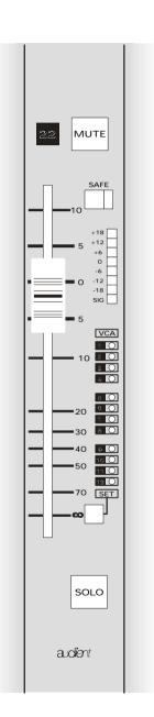
Aztec Input faders are arranged in 8 channel wide panels. There is a single larger panel for the 12 VCA Master faders and the 3 Main Output faders are fitted on the Master output module.
