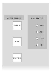
4 LEDs indicate the status of the incoming PSU rails. All Aztec PSUs have on-board switching to allow a second back-up supply to be used.
