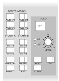
Comprehensive internal assignment of Talkback and Signal generator outputs is provided, along with the ability to send a balanced output to the rearmounted XLR by depressing the EXT button.
