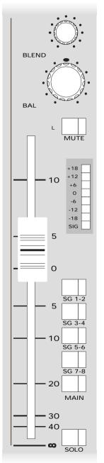
BLEND adjusts the relative levels of signals sent to the L/R and C Main buses.
