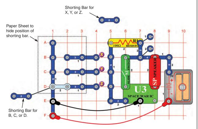
Build the circuit at left. It uses both jumper wires as permanent connections. It also uses two 2-snap wires as "shorting bars".
