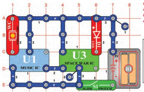
OBJECTIVE: To build a circuit that uses your voice to control a light emitting diode.
