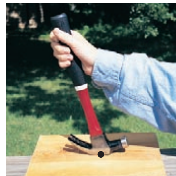
Figure 8-13 A hammer makes it easier to pry a nail from a board by multiplying the input force. The hammer swivels around the point marked with a black dot.
