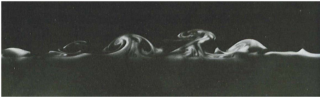
Figure 3.8: Cross-section of a turbulent spot over a flat plate in a wind tunnel. Smoke is used to visualize the spot. Image by Perry, Lim, and Teh, taken from An Album of Fluid Motion , by Milton Van Dyke (1982).
