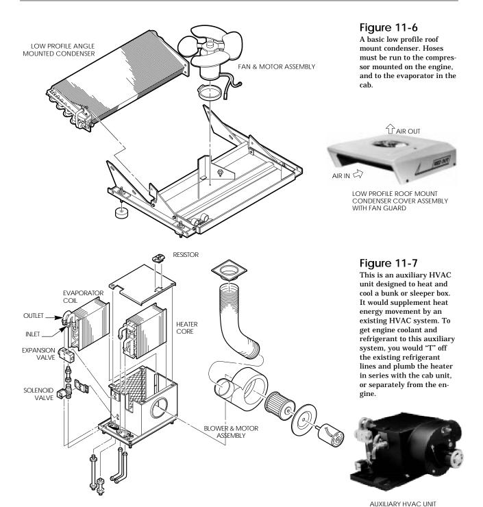
Sleeper cab AC system refrigerant flow is controlled by an electrically operated solenoid valve. The solenoid is wired to the control panel in the sleeper cab. When the operator turns on the bunk AC system, the solenoid valve opens to allow refrigerant to flow to the evaporator mounted under the bunk. With most installations the fan motor cycles on and off to control temperature. Figure 11-8 shows how the sleeper box and in cab AC units may be positioned and connected.
