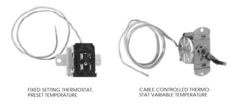
The thermostats shown have sealed capillary tubes that sense temperature. The capillary tubes contain a small amount of heat sensitive gas or liquid like R-12. System temperature variations raise and lower pressure in the sealed capillary tube. This pressure activates a switch inside the thermostat to open and close the electrical circuit to the clutch. These thermostats may sense temperature in the evaporator coil or at the evaporator outlet.
