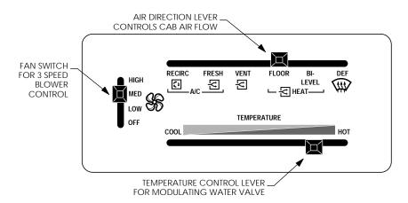
Figure 5-1 HVAC in-cab controls are described in this illustration.
