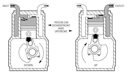
INLET LOW PRESSURE – ON DOWNSTROKE PISTON SUCKS REFRIGERANT GAS THROUGH OPEN VALVE
