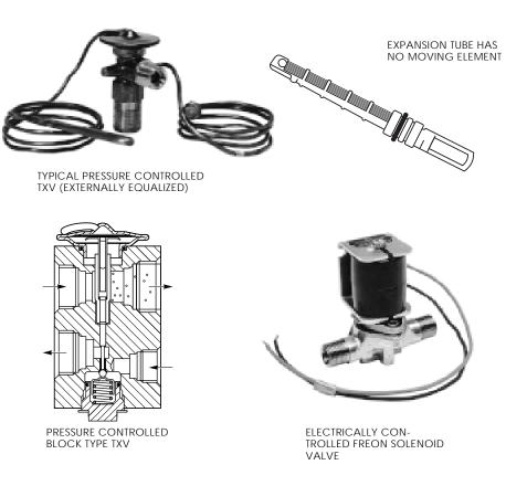
These controls are designed to meter refrigerant flow through the evaporator coil. Thermostat and compressor clutch function are independent of these refrigerant flow control devices.
