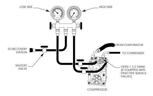
**Note:** The manifold gauges read system pressure when the hand valves are closed if the hose end valves, and the stem type service valves (if included) are open.
