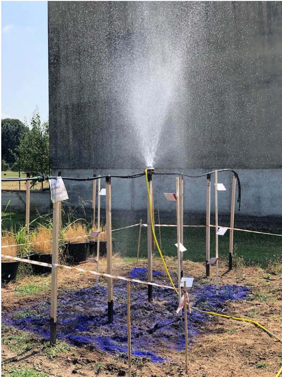
Figure 2. Experiment of rain splashes dispersal on bare soil: artificial rain drops are coloured when touch the ground and the splashes are absorbed by the blotting paper positioned at different heights. Photo credit, dr. Tito Caffi
