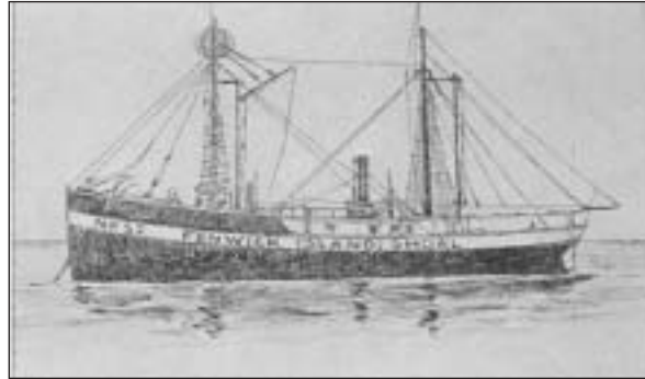
The sister ship, LV-52, assigned to the Fenwick Island Shoal station in Delaware. She had two fixed red lights and a steam whistle.
