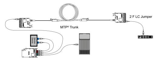
• Configuration B-1: Integrated Tap module with Single Trunk (Interconnect)
