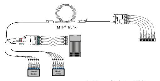
• Configuration A2: Non-Integrated Tap Module with Double Trunk (Cross-connect)
