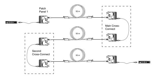
Figure 1: Six MTP-LC Module Links
