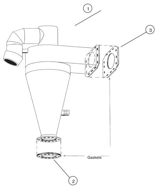
Cyclone U62526 is installed on Vactor® Model 2100 Series Machines (with a fan)
