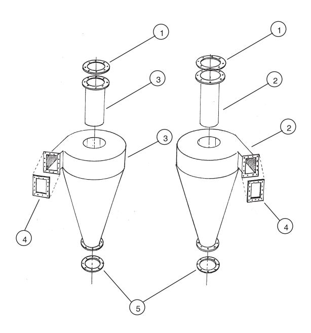
Vactor® 2045 Cyclone Assemblies Manufactured by ASPC
