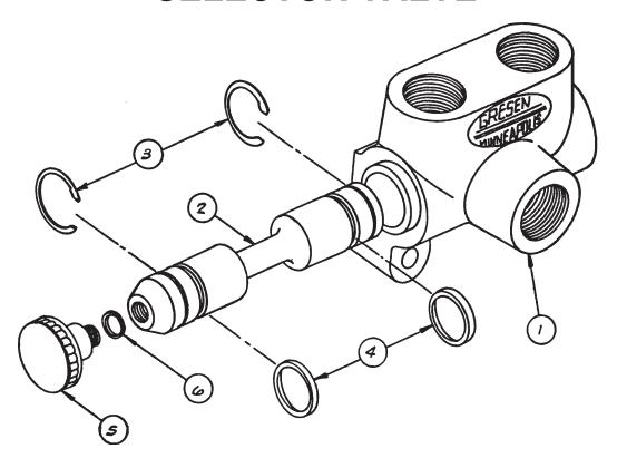
Used on Models 810, 800, 1200 and Early 2100. Operates front hose reel hyd. motor and hyd. hose reel tipping cyc. 60 and 80 GPM reel. Also used on the optional recirculation system.
