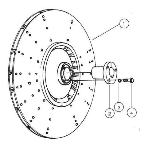
ASPC's own 38" diameter fan assembly are constructed to meet exact dimensional specifications and each part in ASPC's fan assembly is coated with a protectant to ensure long life.
