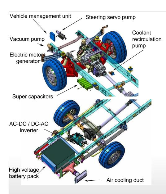
The Daily's 2.3 litre 116 cv (85 kW) Diesel engine (not shown in the picture) works in conjunction with the 44 cv (32 kW) electric motor-generator
