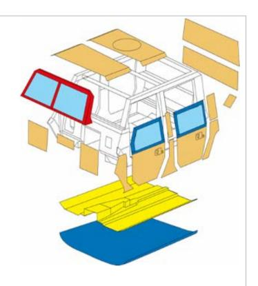
LMV's protection strategy is based on energy management – providing effective absorption or dissipation of energy.
