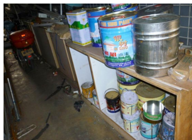
Poor storage of flammable liquids.
