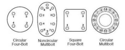
Pass 1 – Tighten nuts loosely by hand in the first instance, according to the cross bolt tightening pattern, then hand-tighten evenly.
