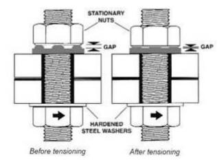
DTI's stay on the job, providing permanent visual and measurable proof that the bolt is correctly tensioned to specification. Gap corresponds to bolt load verified by a test certificate traceable to NIST.
