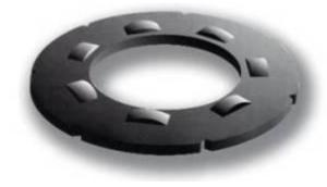
Direct tension indicators provide the means to measure bolt tension (bolt load). They are manufactured as per ASTMF959 and F959M. They are generally used with structural fasteners. The Direct Tension Indicator (DTI) is a specially hardened washer with protrusions on one face. The DTI is placed under the bolt head or nut, and the protrusions create a gap. As the bolt is tensioned, the clamping force flattens the protrusions, reducing the gap.
