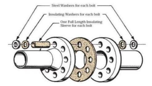
Flange insulation sets comprise the following components which ensure that full electrical isolation is achieved.
