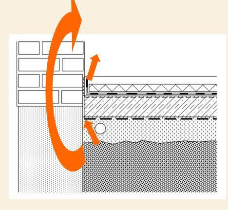
Additionally applied RPI must be connected in an airtight manner to the existing waterproofing below the walls
