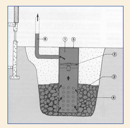
Arrangement of a Swedish radon well:
