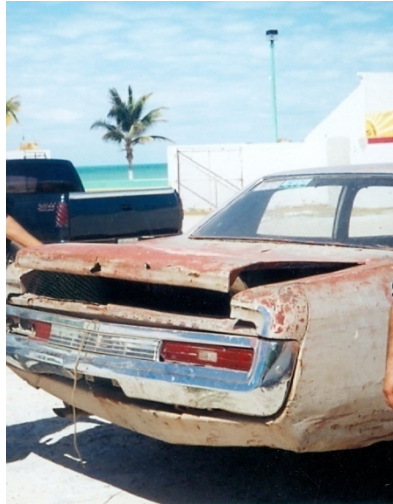
Figure 10. Corrosion on a bodywork exposed to the Gulf of Mexico tropical coast.
