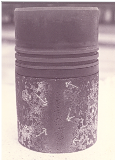
Figure 12. Corrosion in a carbon steel jacket on the water face in a diesel combustion engine truck.
