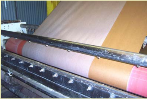
Rod coating of 42# linerboard at Spectra-kote
