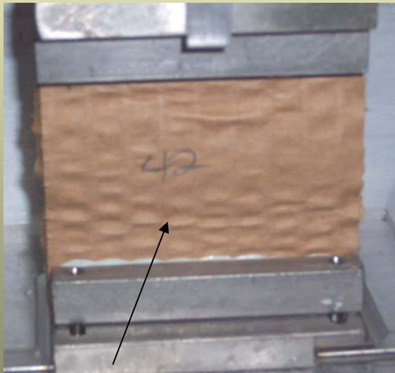
An ECT creep test in cyclic humidity
