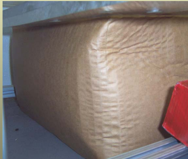
Test box in a cyclic humidity creep test
