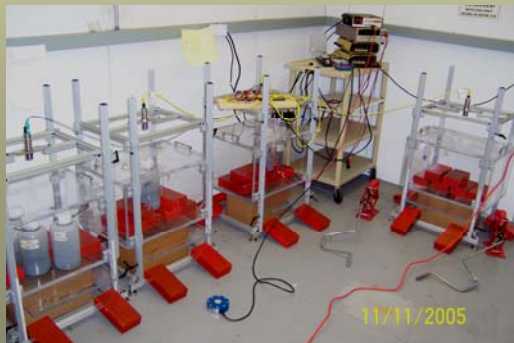
Test boxes put through performance tests, e.g. lifetime in cyclic RH
