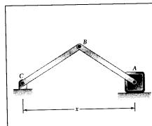
The acceleration of slider A is defined by the relation  $a = -2k\sqrt{k^2 - v^2}$ , where a and v are expressed in ft/s<sup>2</sup> and ft/s, respectively, and k is a constant. The system starts at time t = 0 with x = 1.5 ft and v = 0. Knowing that x = 1.2 ft when t = 0.2 s, determine the value of k.
