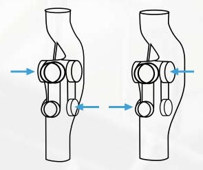
The maximum distance between two Aerators is recommended not to exceed 6m. however, in case of installations with distances more than 6m, it is recommended to make speed reduction loop by using four  $45^{\circ}$  elbows as demonstrated in the below sketch:
