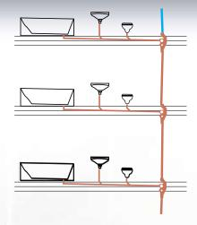
Cosmoplast Aerator has 2 front connections and 4 side connections, all can be used simultaneously. Installations which enables cross flow are not allowed and should not be used, as demonstrated in the below sketches:
