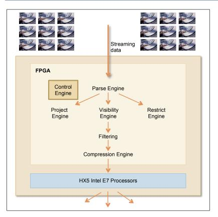
Figure 11: PureData System for Analytics S-Blade Structure
