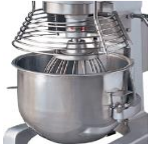
Figure 6- Mixer Safeguard used for safety
