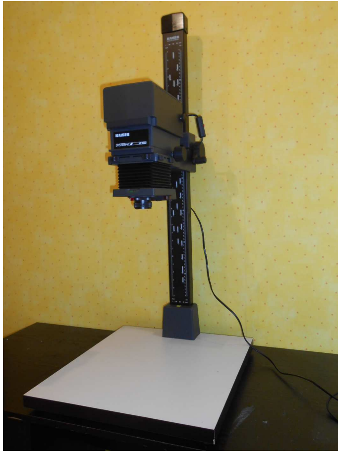
Figure 4: Kaiser B & W enlarger with 80mm lens
