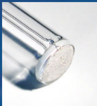
Current generator „electrode“ for cell with diaphragm
