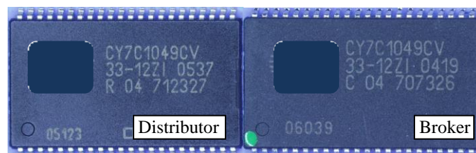
Figure 1 – Comparison of two SRAM parts. Different lot numbers.
