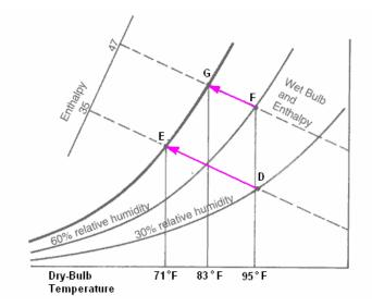
Evaporative cooling process with hot dry air from points D to E and with hot humid air from points F to G. Notice greater evaporative cooling capacity with dry air.
