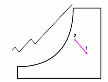
The evaporative cooling process is commonly employed to reduce the dry bulb temperature of the air without refrigeration. It is a constant wet bulb process of reducing dry bulb temperature. The hardware used to achieve this process usually consists of the basic components of the adiabatic saturation chamber plus some type of device to amplify the interface surface area between the water reservoir and the air, such as wetted wick, matting, plates, spray, etc.
