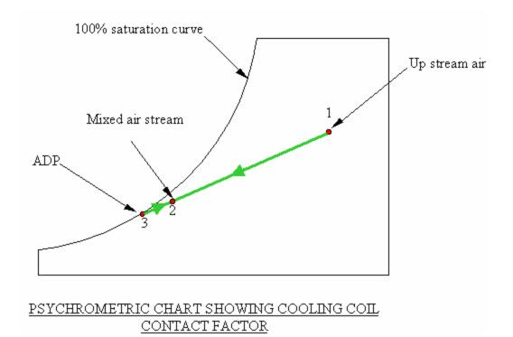
The air that does not come in contact with the cooling coil is the "bypass factor" (BF) of a cooling coil may be found from;
