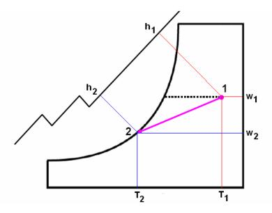
On psychrometric chart, this process is represented as line sloping downward and to the left. This process is assumed to occur as simple cooling first and then condensation. While the moisture is condensing the air is assumed to remain saturated.
