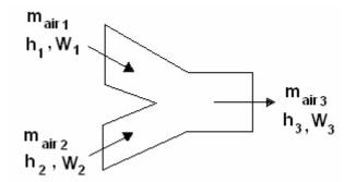
In most cases, heat loss from the system is negligible and the system can be modeled at adiabatic. On a psychrometric chart, the condition of the exiting air stream must be on the line connecting the incoming air streams. The distance along that line is determined by the ratio of the mass flow rates of the incoming streams.
