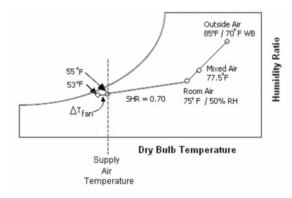
Determine enthalpy for coil entering and leaving conditions
