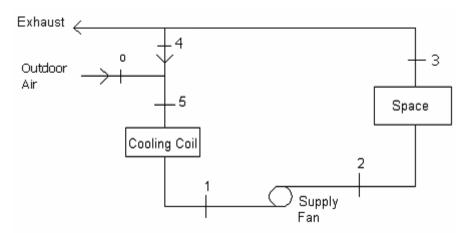
Simple Schematic of Cooling Unit
