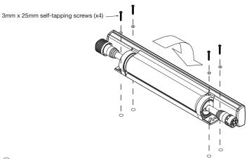
Rotate fixture to gain access to mounting holes.
