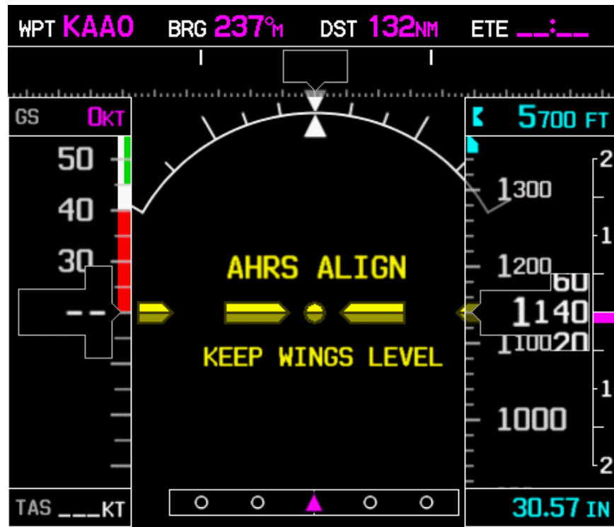
Figure 10-4 – AHRS Align Message (PFD)
