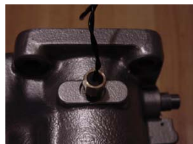
Figure 8-19. Carb Temp Sensor Installed
