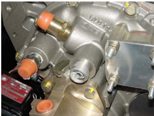
Figure 8-11. Tachometer Drive Output
