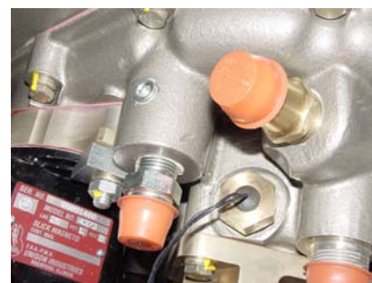
Figure 8-10. Oil Temperature Probe Installed (Crush Gasket Not Shown)
