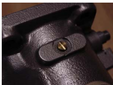
Figure 8-17. Carb Temp Sensor Mounting Location
