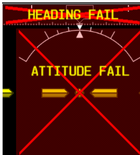
Figure 10-6 – Attitude and Heading Failure Indications (Reversionary or Split-Screen PFD)
