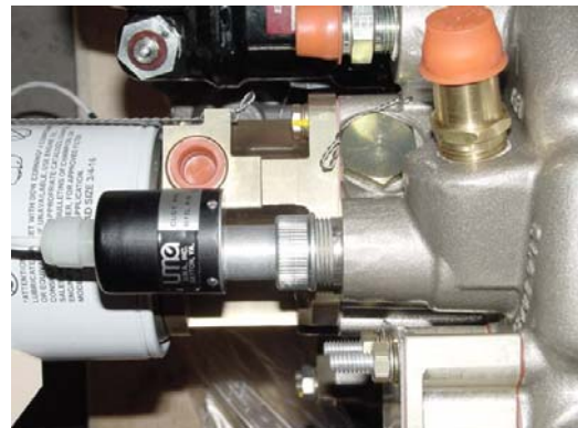
Figure 8-12. Installed Tachometer Sensor
