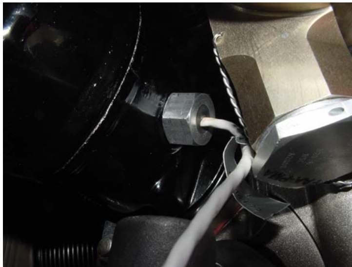
Figure 8-14. Magnetic Tach Sensor Installed
