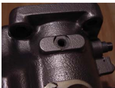
Figure 8-18. Carb Temp Sensor Mounting Location w/ Screw Removed
