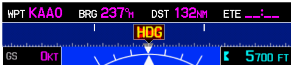
Figure 10-5 – Heading Failure Indication (Full-Screen PFD)
