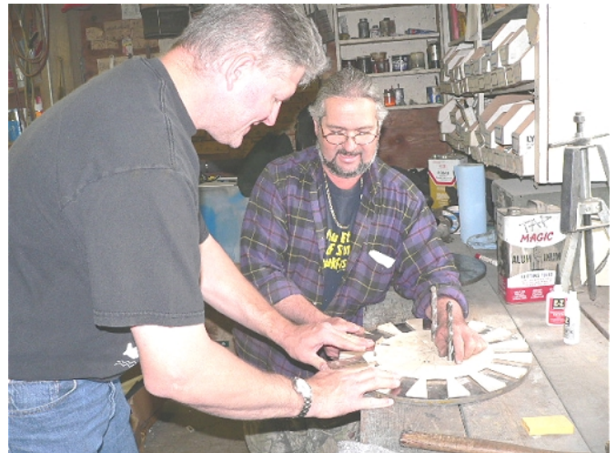
Instructor George chuckles while Jay places a big magnet on one of the 15 foot machine's big magnet rotors. The magnet placement template makes a nearly impossible task easy. The template is removed before resin is poured in to cast the magnets in place.
