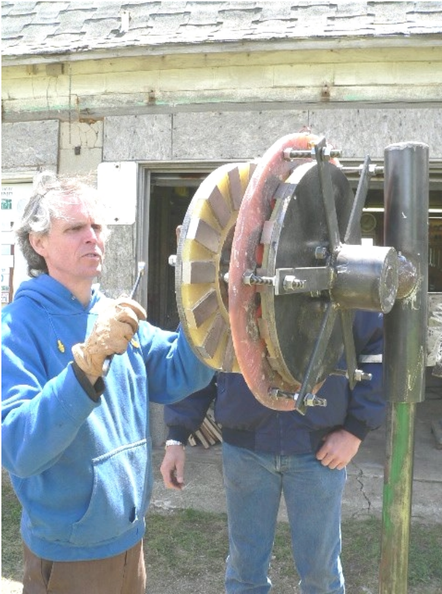
DanM shows the proper look of intense concentration while slowly lowering the front magnet rotor into place on the big 15 foot machine with the jacking screws
