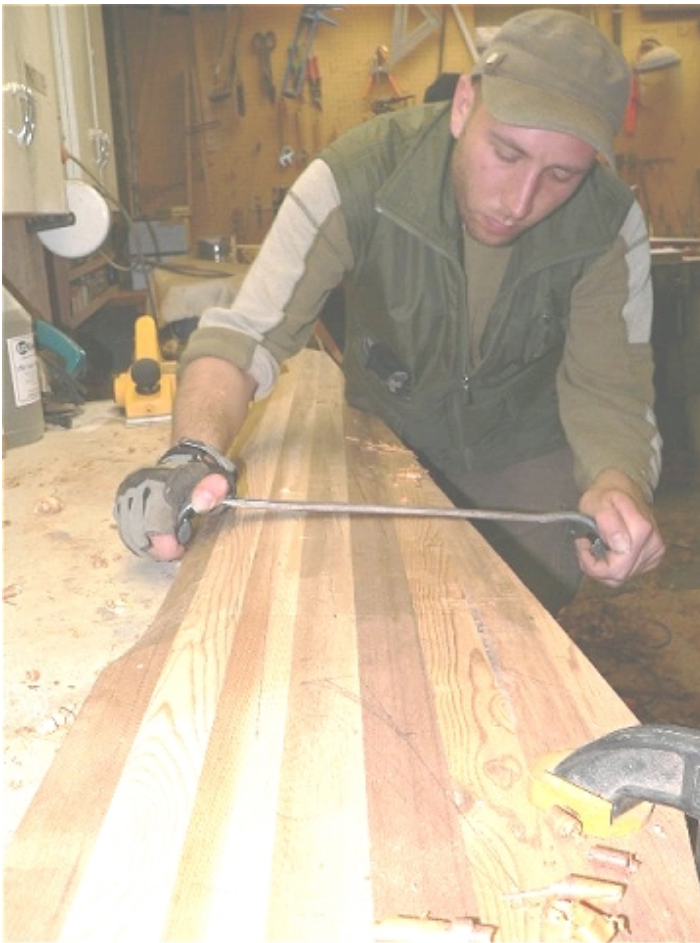
Josh from the MREA carves the airfoil on the back of the blade with a drawknife. Anyone who starts making blades will quickly become a 'connoisseur' of drawknives. Bad ones make your life miserable.
