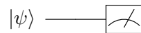
FIGURE 4.6: Symbol for projective measurement on a single qubit. In this circuit nothing further is done with the measurement result, but in more general quantum circuits it is possible to change later parts of the quantum circuit, conditional on measurement outcomes in earlier parts of the circuit. Such a usage of classical information is depicted using wires drawn with double lines.
