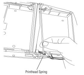
4. Slide and lift out the printhead assembly. See Figure 42.
