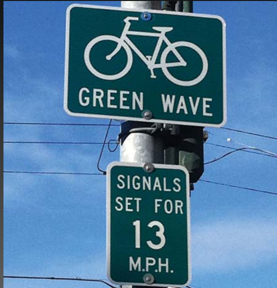
Figure 15. NACTO "Green Wave" – Coordinated signals on corridor with bicyclist prioritization
