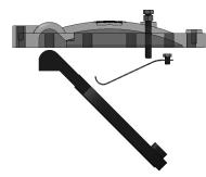
Neatly tucked behind the disc, it accelerates closing speed, reduces water hammer and never interferes with flow.
