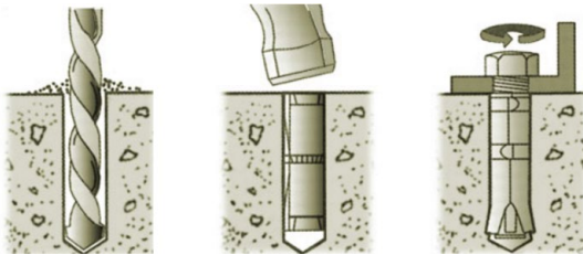
Figure 3-8 Drill holes, set Anchors, and tighten Assembling Bolts
