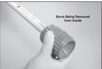
A slight bevel must be placed at the end of the pipe, as shown below. A slight bevel will ease the entry of the pipe into the socket and minimize the chance of cement being wiped off the fitting.
