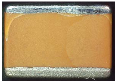
e) Cracking caused by manual soldering.
