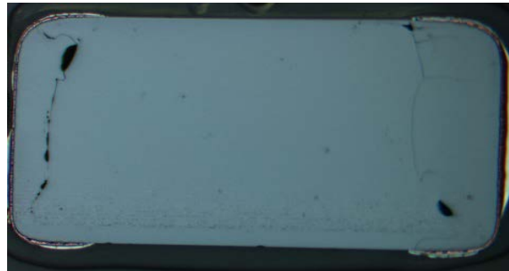
d) Assembly-related defect: thermal shock cracking.
