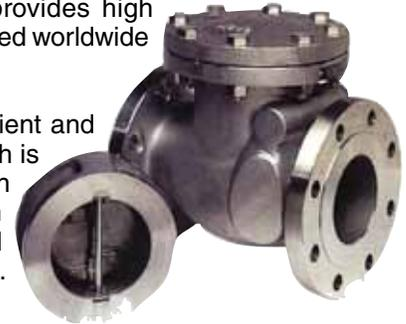
The Duo-Chek® also offers special design features that make it a high performance non-slam check valve. These include a scrub-free opening, and in most sizes a unique independent spring design as well as an independent plate support system. These features may not be found in other check valves. Other configurations offered include lug, double flange and extended body.
