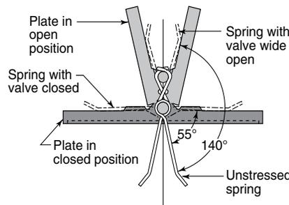
A spring design of the Duo-Chek® (sizes 6" and larger) allows higher torque to be exerted against each plate with independent closing in response to the process stream. Testing has proved this action provides up to 25% improvement in valve life and 50% reduction in water hammer.
