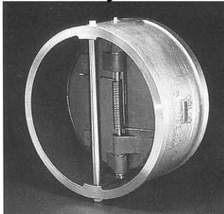
The Style X body design has special geometry and plate configuration to allow each plate to strike the stop pin in its center of percussion. To absorb high impacts, the stop pin and hinge lugs are oversized.
