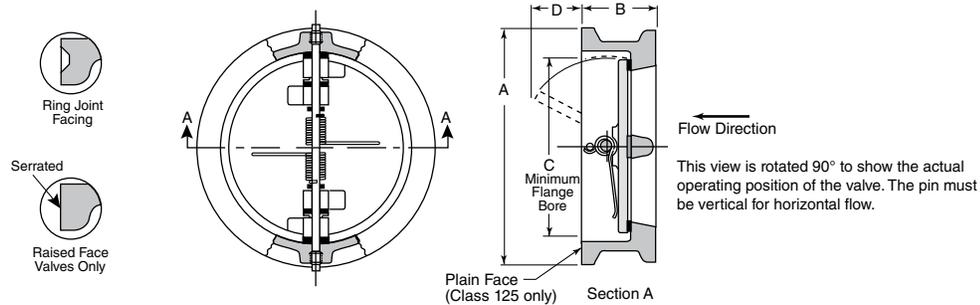
Wafer body valves are designed with flangeless bodies with short face-to-face dimensions per API 594. They are clamped between mating flanges which are connected by studs and nuts.
