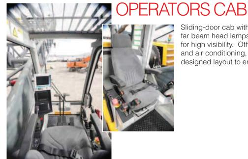
Sliding-door cab with large area windows, near and far beam head lamps, and rear-view mirrors allow for high visibility. Other features include heating and air conditioning, MP3 player, and ergonomic designed layout to ensure operator comfort.
