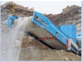
The discharge product conveyor is dust sealed. Dust filter or water spray nozzles in the crusher and on this conveyor are options.
