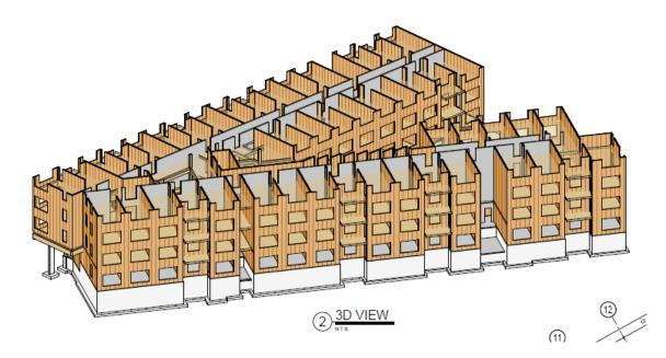
Figure 6. - 3D view of 340 structure from Orchard Street. Credit: Odeh Engineers
