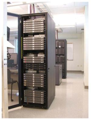
Illustration 5: Rack of 30 1-U servers. Note the boxes of KVM switches above each cluster of six servers. The bottom three servers in the middle cluster have their escutcheons removed to allow access the optical drives and USB ports.
