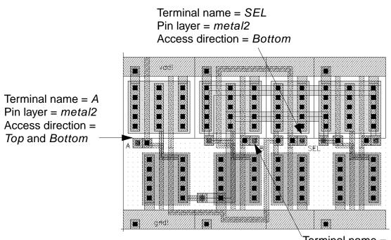
Terminal name = BPin layer = metal2Access direction = Bottom
