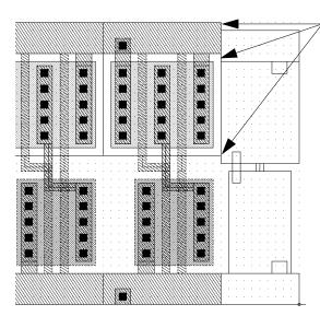
The inverter does not align with the nand.
