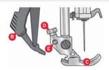
Squeeze the Dynamic spring foot 6D gently together and guide the pin of the foot into the cross-hole (E) of the presser foot holder as far as it will go. The arm on the foot should be placed behind the needle screw.
