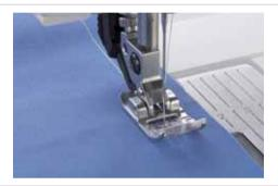
Piecing with a  $\frac{1}{4}$ " (6mm) seam allowance using the Quilting Foot with IDT<sup>TM</sup> system
