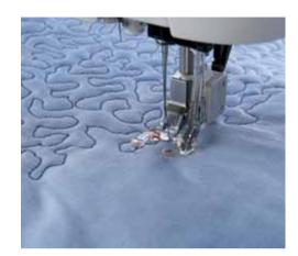
Touch Sensormatic free-motion setting to set the machine for Sensormatic free-motion mode with presser foot 6A.
