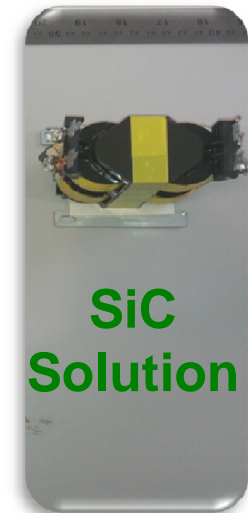
Transformer at 100 kHz
