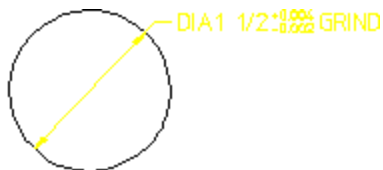
Figure 99. Combining Dimensioning Commands and Functions
