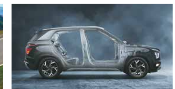
Strong body structure with AHSS
