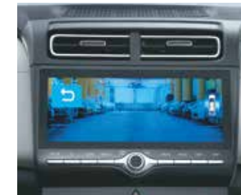
Driver rear view monitor
