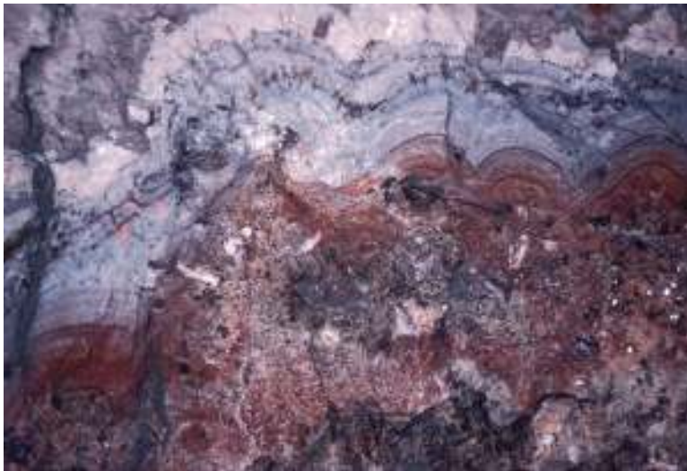
Figure 15.4 Banded aplite ore from the Tanco deposit. Tantalum mineralisation is contained in the banded aplite (red and blue-grey at the bottom). A massive quartz zone (dark grey) is at the top and coarse, crystalline white beryl separates the aplite and quartz. The scale is approximately 2 m across. (Courtesy of R. Linnen.)
