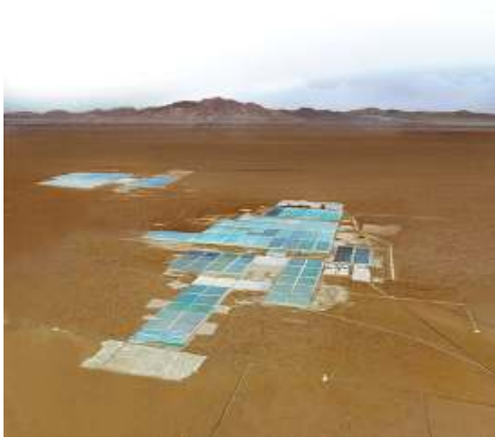
Figure 10.5 SQM's solar evaporation pond system at the Salar de Atacama covering an area equivalent to 7000 football pitches and in excess of 30 km 2 . (Photograph courtesy of Sociedad Quimica y Minera de Chile S.A. (SQM).)
