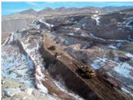
Figure 5.8 Materion Brush open-pit mining at Spor Mountain, Utah. (Courtesy of Materion Corp.)
