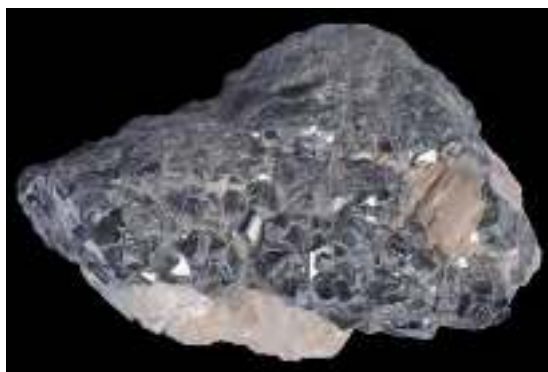
Figure 6.1 Skutterudite, a cobalt–nickel arsenide, from Bou Azer mine, Morocco. Maximum dimension of specimen is 7 cm. (BGS © NERC.)
