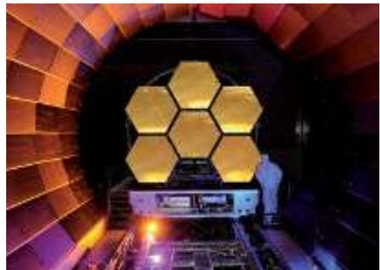
Figure 5.2 Six of the 18 mirrors of the James Webb space telescope undergoing cryogenic testing at the Marshall Space Flight Center, Huntsville, Alabama, USA. (Photo: K. Hutchison, courtesy of Ball Aerospace and Technologies Corp.)
