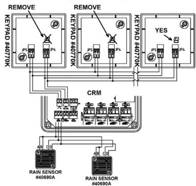
Example B-1: Using Multiple Keypads with one CRM
