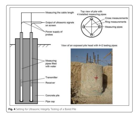
the position of the joints should also be recorded. Steel pipes with welded caps and crimped connections have proved effective.
