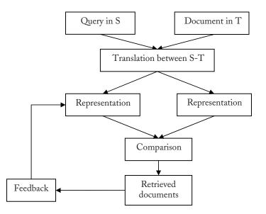
FIGURE 1.3: Typical architecture of a CLIR system.
